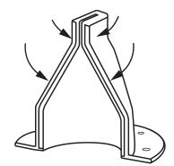
...reverse pressure seals the valve closed, even on solids, to prevent backflow into the process line.
