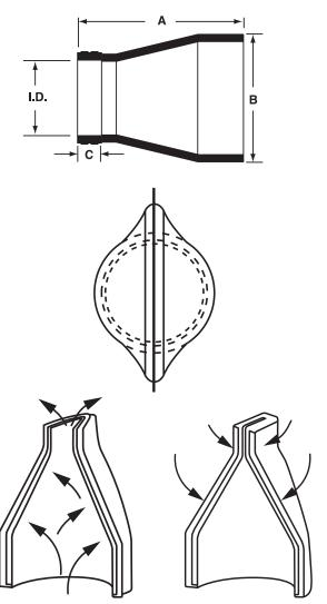
The FlexValve® 4100 check valve opens with line pressure to allow the process media to flow through...
