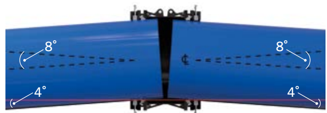
4° Angularity across the range at both ends
